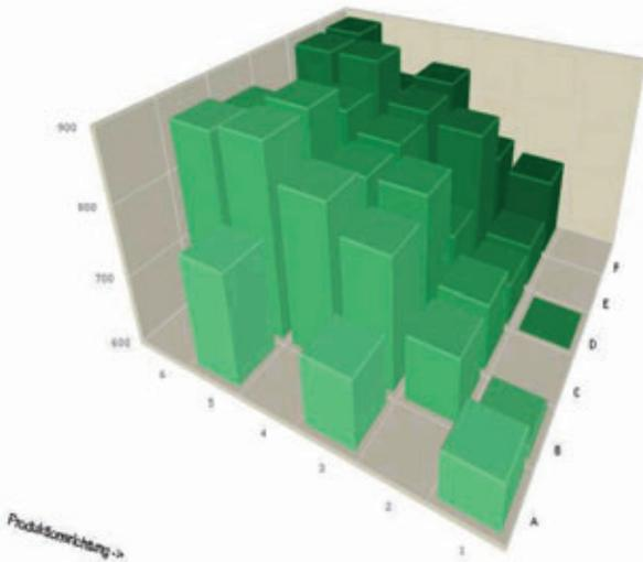
Fig. 4a: Example display of uneven quality of compaction of the core concrete on a production board
