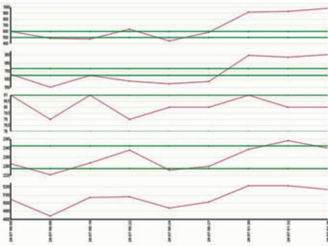
Fig. 3: Example display of all five measurements from a production with large fluctuations in quality (the red lines each represent the connected 9 measurement points) over the time axis with tolerances (green lines). From top to bottom in the display: 1. Compaction of facing concrete, 2. Compaction of core concrete, 3. Height of the product, 4. Gross density of the product, 5. Weight (without limit lines)
