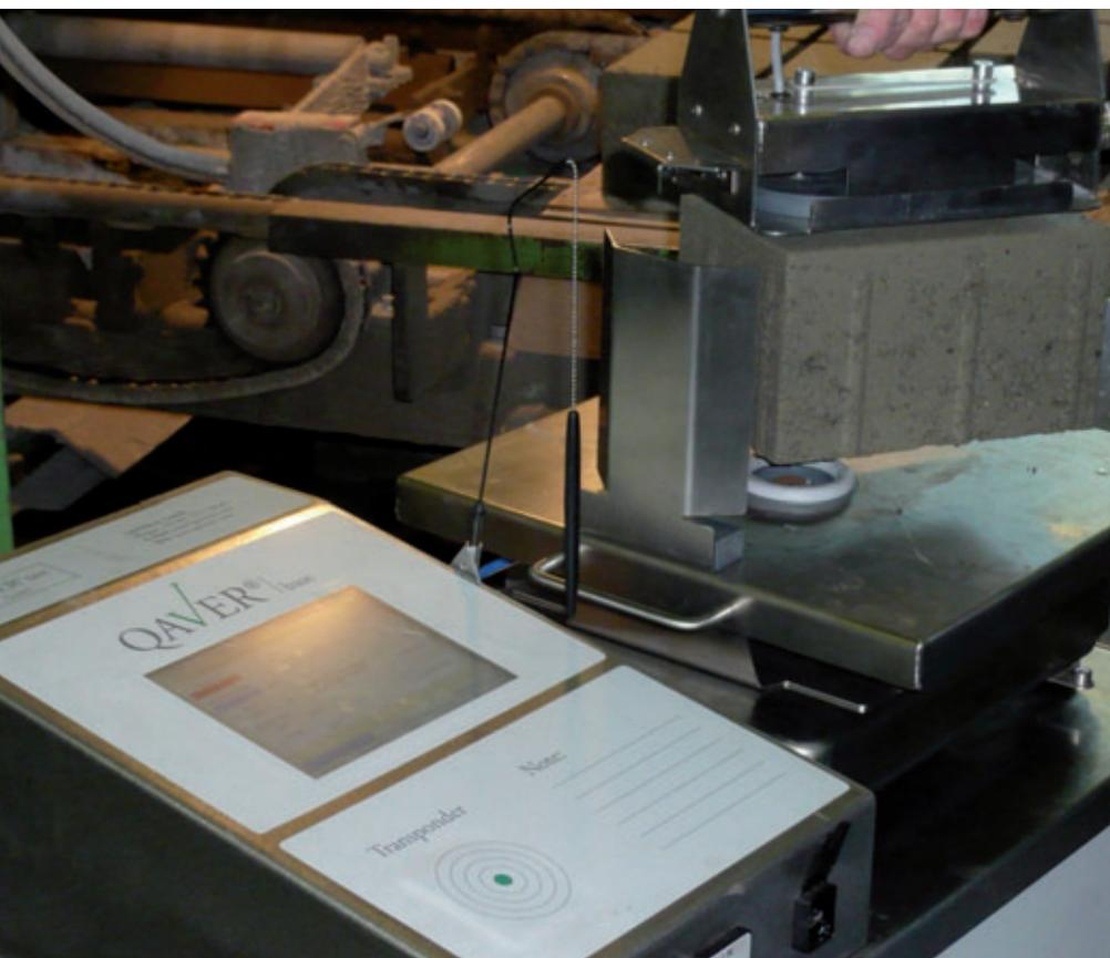
Fig. 1: The Qaver is placed directly on the plant and requires only a 220 V supply for operation. The lifting device enables paving stones to be lifted to a height of 140 mm or a weight of up to 12 kg. Various types of suction cup are available for different surface properties.
