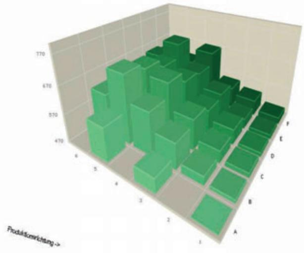
Fig. 4b: Display of the quality of compaction of the facing concrete on the same board
