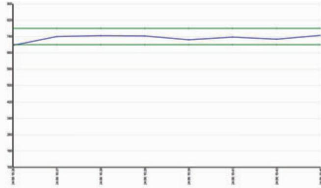
Fig. 2: Example display of the compaction quality of the core concrete from an even production over 8 measurements. The blue line shows the connected measurement points. The green lines mark the limit range of the tolerance entered in the Qaver for the product.
