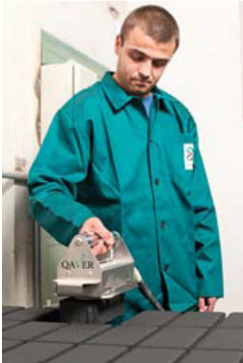
Fig. 2 Removal of a freshly manufactured concrete product for quality testing with the Qaver.
